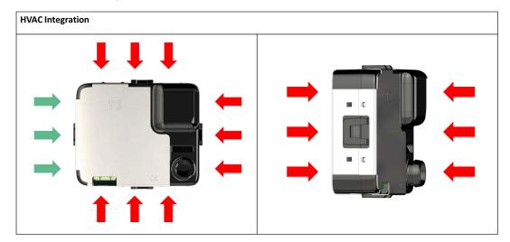
Be aware that it is not recommended to place the inlet of the NextPM in an opposite direction with the airflow of the HVAC system.
