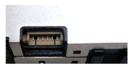
The connector is a 6 PIN one. You can use an ADAM TECH 125CH-B-06 reference to connect with or an equivalent like a MOLEX 51021-0600 reference.
