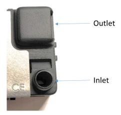
The sensor uses an active airflow to sample the particles. In order to keep his accuracy, we advise you to put the inlet directly to the air you want to monitor. If the integration is difficult, you can add a duct made with antistatic materials and with an internal diameter of 8 to 9 mm. The maximum length of the duct must be 100 cm.
