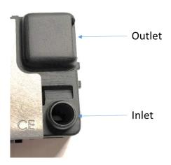
The sensor use an active airflow to sample the particles. In order to keep his accuracy, we advice you to put the inlet directly to the air you want to monitor. If the integration is difficult, you can add a duct made with antistatic materials and with an internal diameter of 8 to 9 mm. The maximum length of the duct must be 100 cm.
