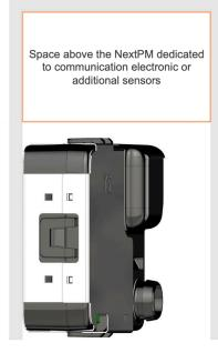
A bottom open system is also possible for the NextPM integration. The larger the opening, the better the sensor will operate.
