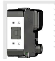
The casing with louver is a good option for outdoor air PM monitoring. It allows a good ventilation of the air inside the casing to be sure that the pollution is the same inside the casing and outside. It prevents the NextPM sensor from rain, and does not expose the sensor to direct sunlight. Moreover, the inlet and outlet are at the same pressure.
