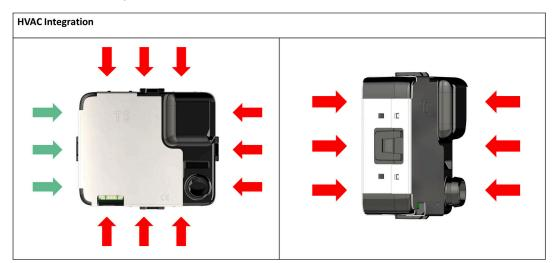
If you can't place the sensor into the airflow directly, the main concern you have to mind is that the inlet and the outlet of the NextPM must be set at the same pressure. The sealed casing presented in the general integration tips can be used.
