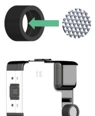
To extend the lifetime of the device, we recommend placing a metallic grid at the inlet of the NextPM to avoid insects or dust getting in the sensor. A cap including the grid can also be provided by Tera Sensor to correctly set the grid at the NextPM inlet (please contact support@groupe-tera.com for further details).
