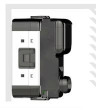
The casing with louver is a good option for outdoor air PM monitoring. It allows a good ventilation of the air inside the casing to be sure that the pollution is the same inside the casing and outside. It prevents the NextPM sensor from rain, and does not expose the sensor to direct sunlight. Moreover, the inlet and outlet are at the same pressure.
